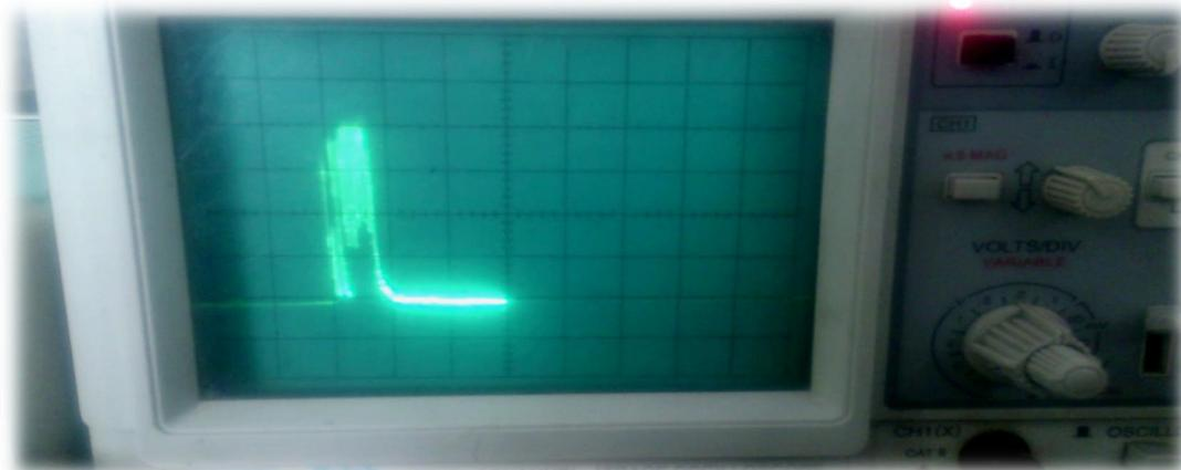
When all the crystals are pressed together at a time with the help of piezoelectric platform it generates peak voltage of 40volts for 5milliseconds.
