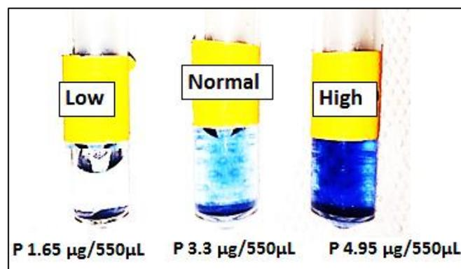
**Figure 1: Standard aqueous Phosphorous solutions and their respective colour differences**
