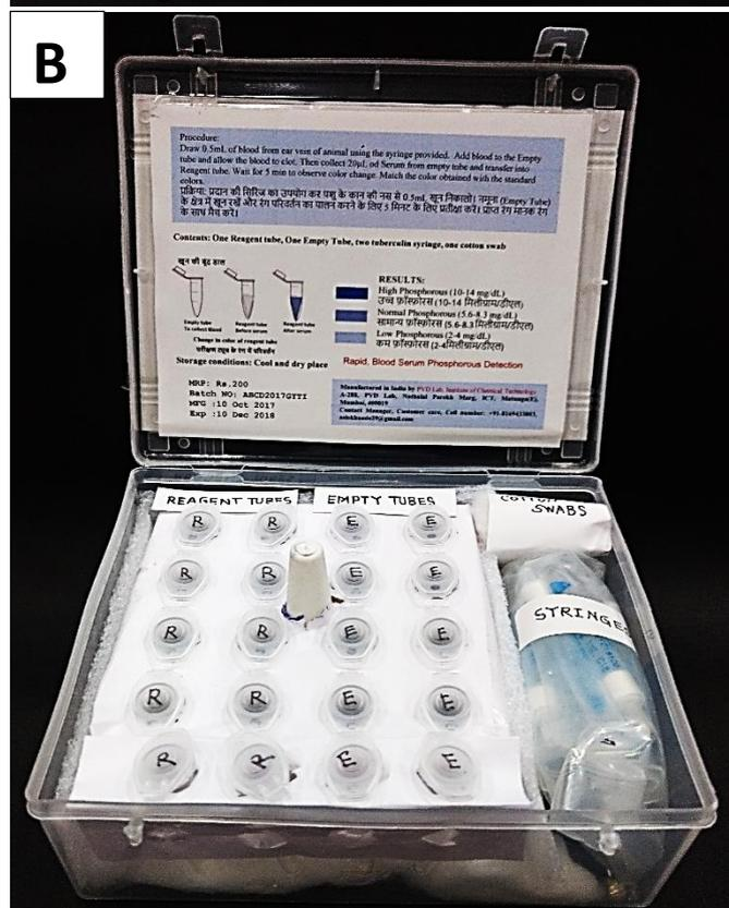
Phosphorous Detection Kit assembly (A) Front View, (B) Inside View
