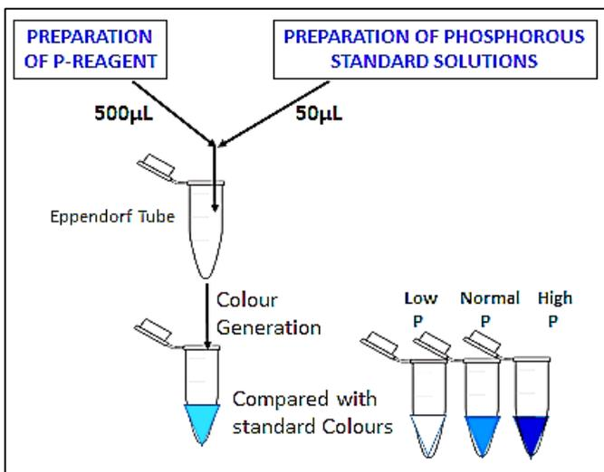
Figure 2: Flow sheet for Phosphorus Detection
